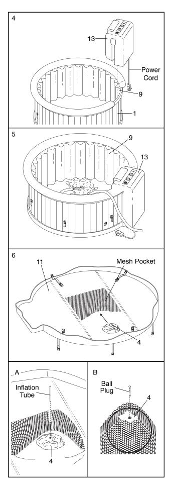
Place the Spa Cover (11) over the Side Panels (1, 2) and the Spa Jet Unit (13). Be sure that the Spa Cover is properly centered and that the straps on the Spa Cover line up with the straps extending from the slots in the Side Panels (1, 2).
